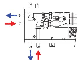
Electrothermal actuator can't be installed in the body of the trench heater due to limited internal space
