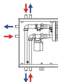
Electrothermal actuator can't be installed in the body of the trench heater due to limited internal space.
