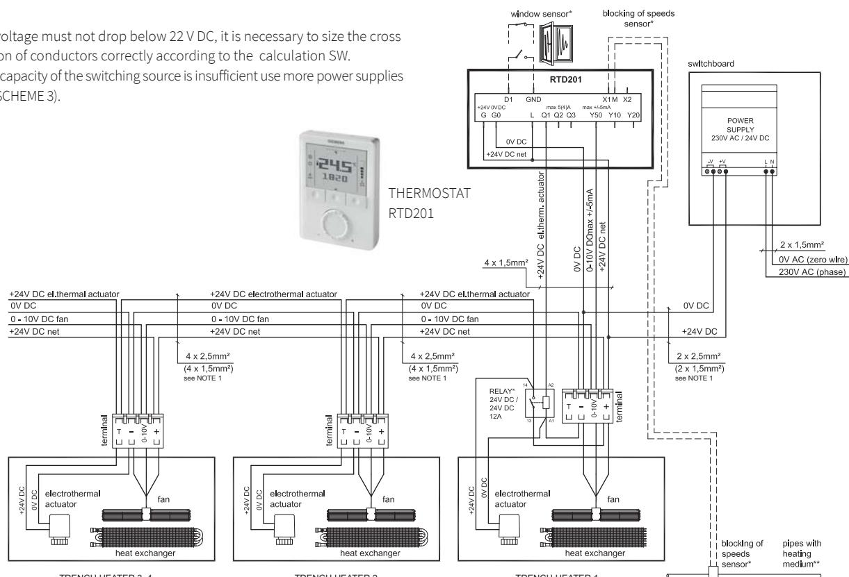
\*accessories / \*\* The temperature sensor (block of revs) must be fixed on the tube, through which the heating medium freely flows and which is not closed by the actuator.
