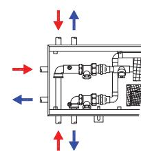
Electrothermal actuator can't be installed in the body of the trench heater due to limited internal space.
