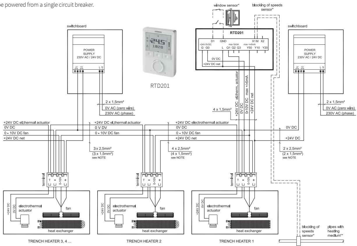
\*accessories / \*\* The temperature sensor (block of revs) must be fixed on the tube, through which the heating medium freely flows and which is not closed by the actuator.
