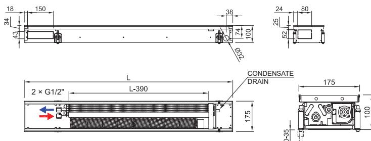
**Warning:** When a **condensate pump** is used, the trench heater is **200 mm longer**. If a pump is required, this should be stated in the order. **Lengths: 1 000; 1 400; 1 800; 2 200; 2 600 and 3 000 mm.**
