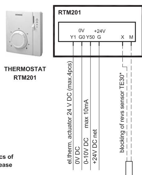
Note: Thermostat RTM201 can control only 4 pcs of electrothermal actuator, for more pieces use please relay RL10, connection by Scheme 2
