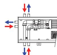
Electrothermal actuator can't be installed in the body of the trench heater due to limited internal space.
