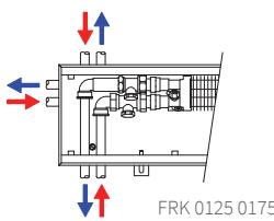
Electrothermal actuator can't be installed in the body of the trench heater due to limited internal space.
