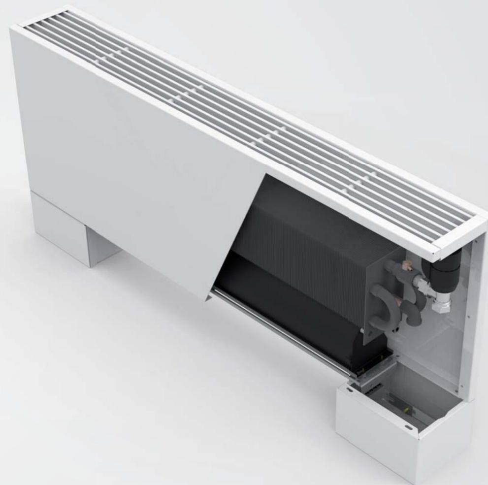
Low surface temperature convectors with lamellar heat exchanger are modern heating elements used for offices, commercial areas, car showrooms, hotels and other public buildings. ECOLITE convectors are suitable for rooms which need thermal screening of large glassed-in panels, e.g. French windows, shop-windows or walls exposed to cold air impact.
